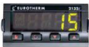
Over-temperature limit controller
